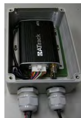
Equipment fitted to cars enabling ASEZA to manage its fleet with a sophisticated Global Positioning System (GPS) tracking system.
