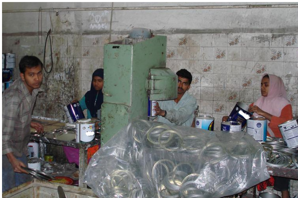
A metal can factory in Amman exhibits disorganized production flow, poor cleanliness and low safety standards.
