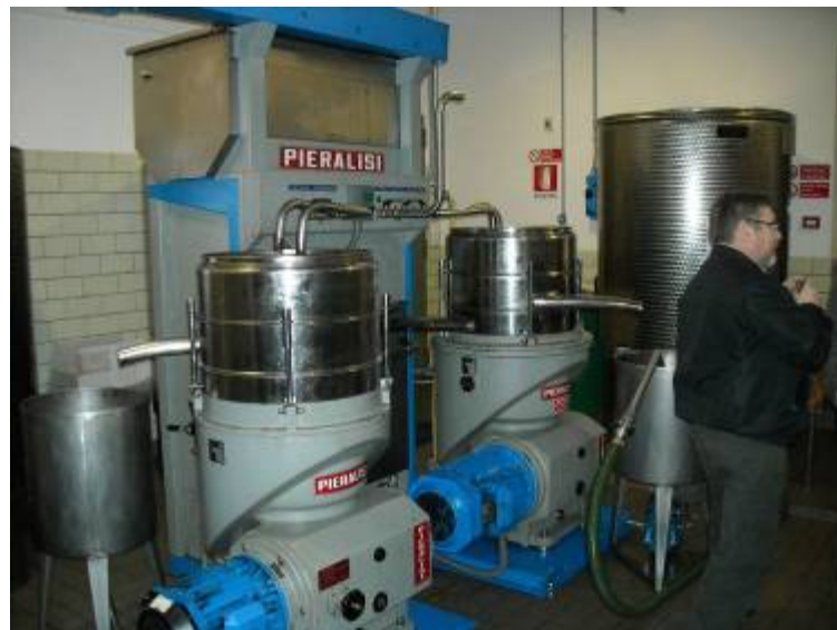
Figure 3. The decanter system at an olive oil plant.
